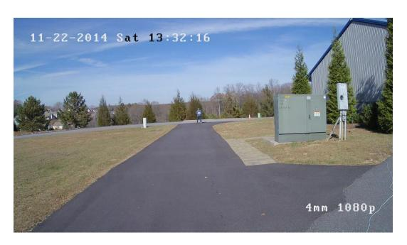
With greater distances, a wide angle view camera will lack the ability to identify faces. It becomes necessary to use a higher millimeter lens when you are trying to identify a security threat that is further away.
