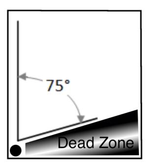
This means that you really need two cameras to cover that area. With one 98 degree camera, you could cover the whole space and not have to buy two cameras (The walls are 90 degrees). So, a varifocal camera, set at 98 degrees would be able to see the whole room.
